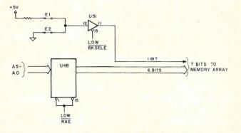
Fig. 3. Address path during Row Address Enable.
